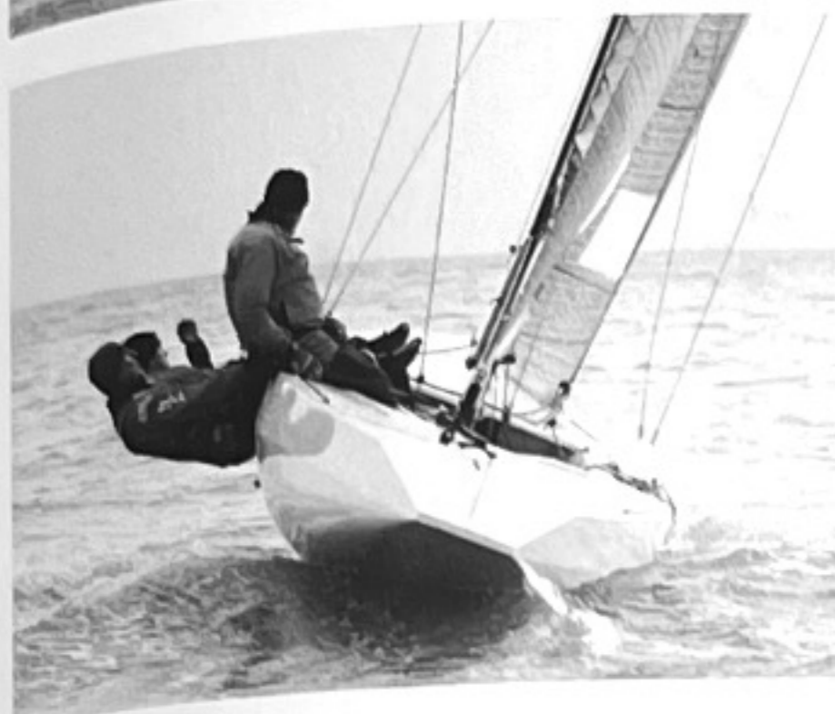
Opposite clockwise: Jean Genie here clearly using all of that long aft overhang – note the narrow upper girths of the mainsail which compromised the use of a thicker upper mast section to do away with runners; the clean and modern cockpit co-designed by Andrew Palfrey and builder Gavin Tappenden incorporates thoughtful Star-style handholds for today's mini-hiked 5.5 crews; IRC-style thick fin keel with a subtle reverse taper, leading-edge 'wedge', large trim tab and small delta-wing endplate... but no wings or ballast bulb. Top: Steve Quigley's own new 5.5 Metre shows a rounded stern while Hollom typically goes all-in with the board-flat approach ( left ). Right: Jean Genie ... showing a smooth-flowing transition from bow U-sections to V-sectioned mid-body and a completely flat run aft
