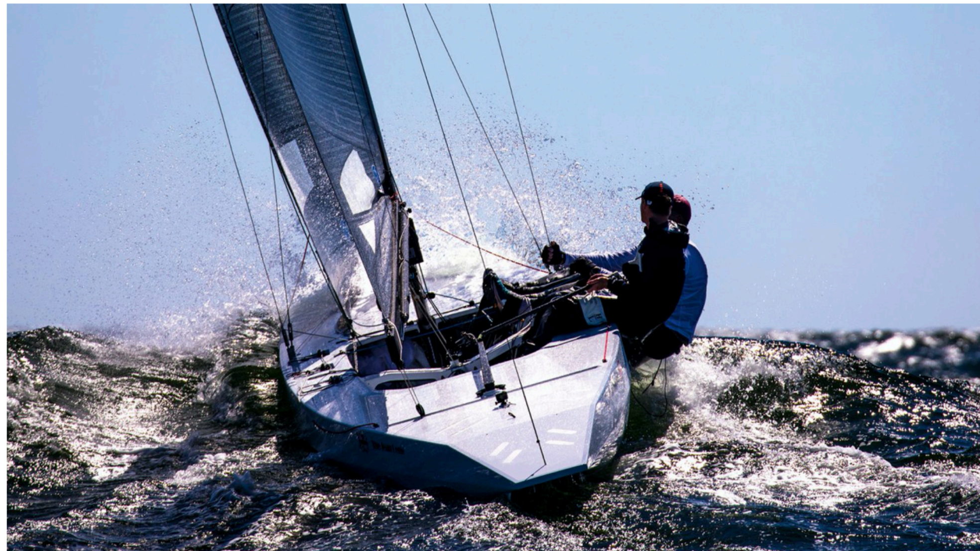
Most 5.5s don't have a mainsheet traveller, but fitting one gave better balance control and helped the team develop more options for upwind modes. Photo: Robert Deaves
