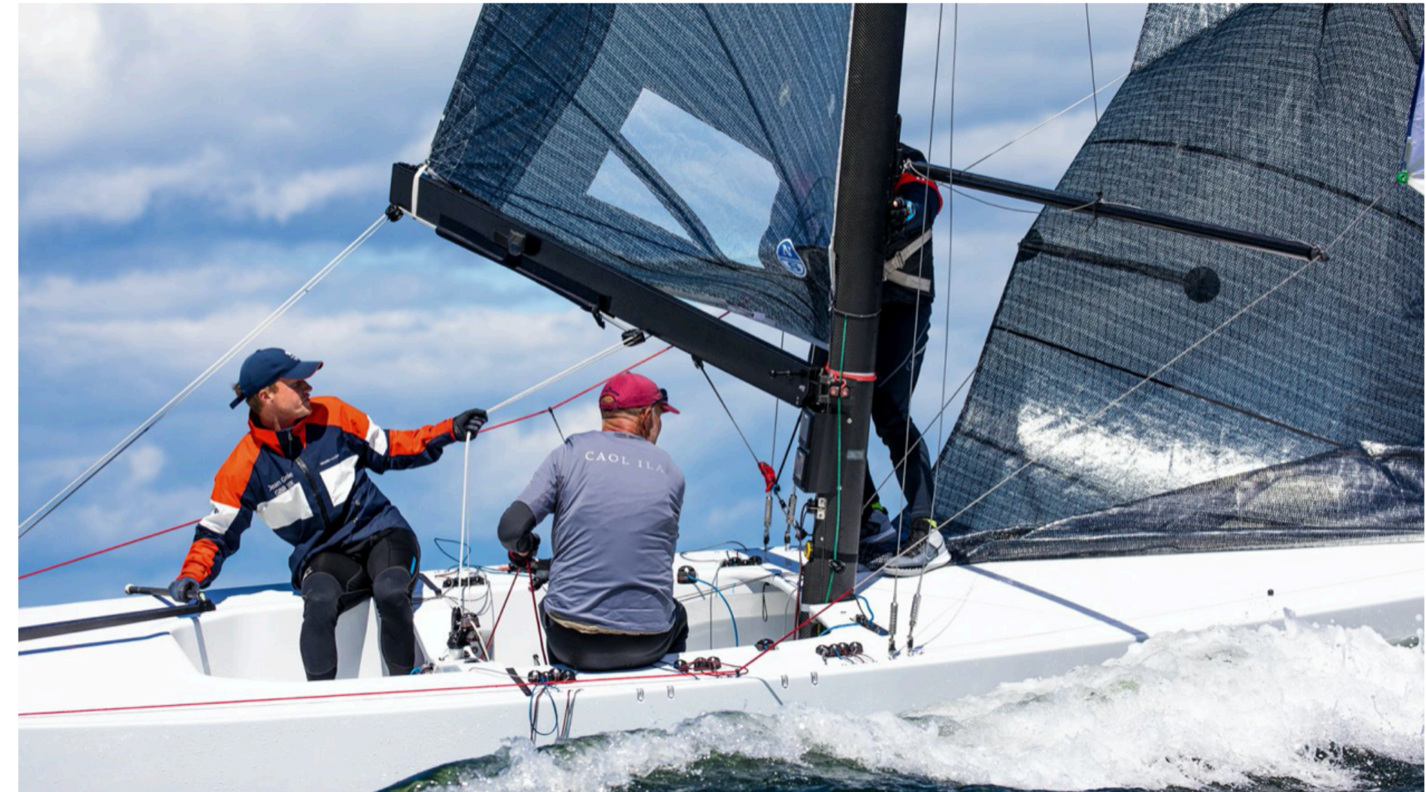
The slightly wing shape mast from Heol Composites has a long chord and is immensely stiff, so running backstays aren't needed. Photo: Robert Deaves
