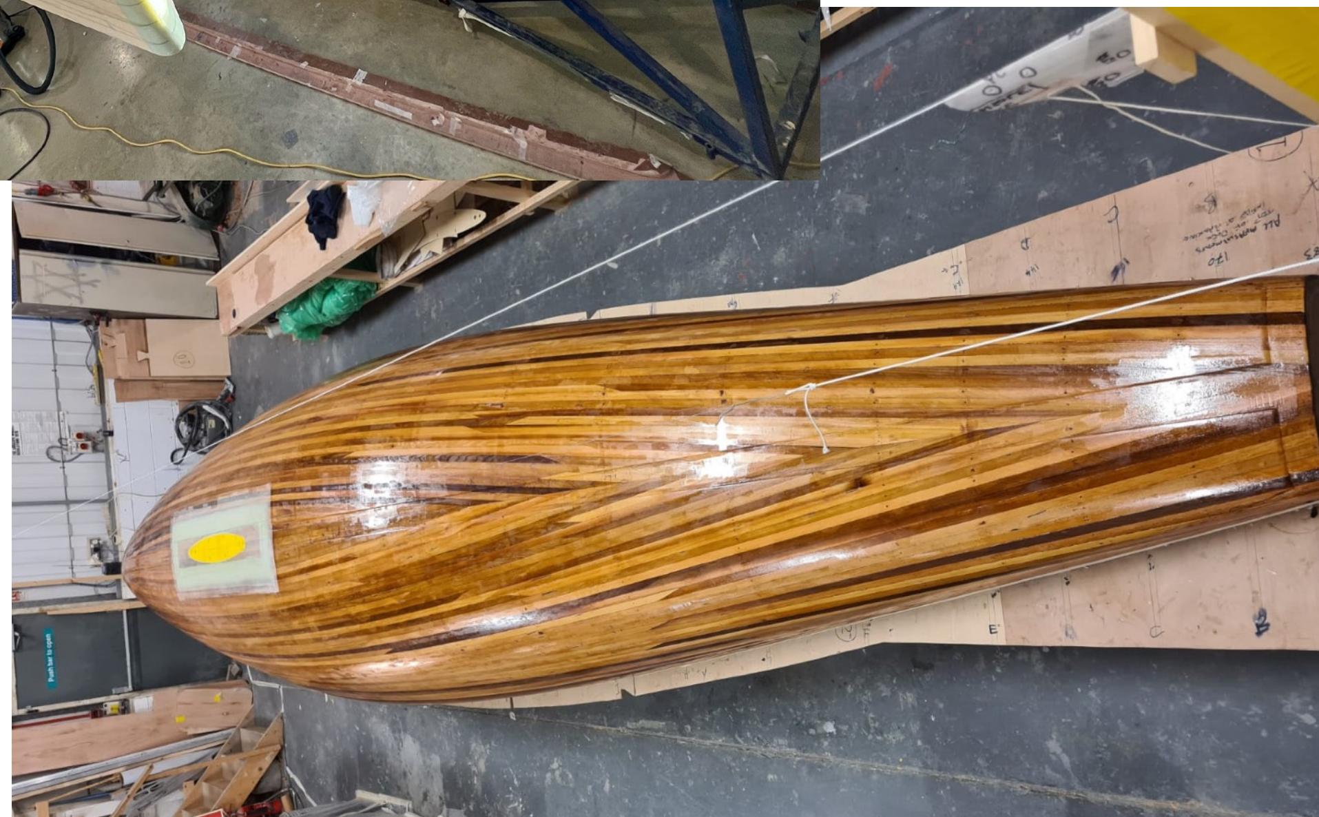
Right: GBR 41, the Quigley designed boat. Cedar planks laid over frames
