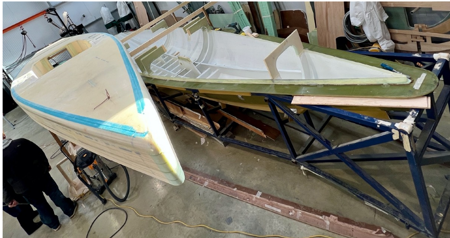
Left: GBR 42. The pre-preg deck and hull about to be joined
